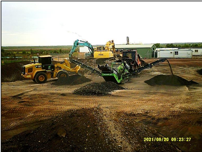
Photo 10. Crushing & Screening asphalt
