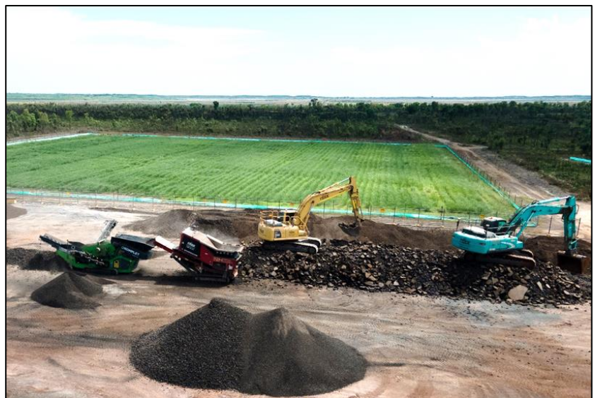
Photo 7. Asphalt crushing & screening process on site
